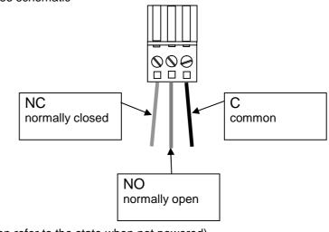
(Note: normally closed and normally open refer to the state when not powered)
