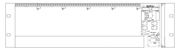
The **AMG2006-DR** Subrack is a dual power feed standard 19" rack-mount subrack. It is designed to house AMG 2000, 2700, 2900 series video transmission equipment.
